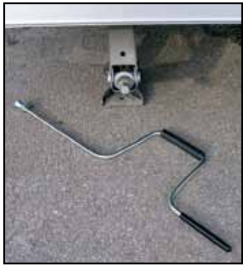
Scissor Jacks are located at each corner of the trailer. Using the crank handle provided, level unit from side to side.
