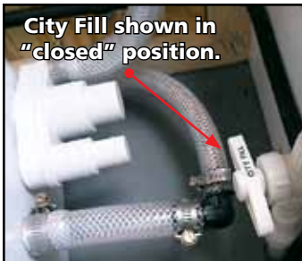
It is recommended that the City Fill valve be in the "closed" position while using the On-Board Fresh Water System.
