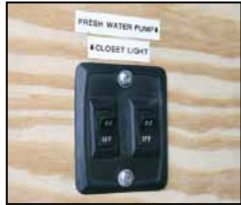
Demand pump power switch.
