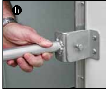
Fasten railing to trailer at bracket.
